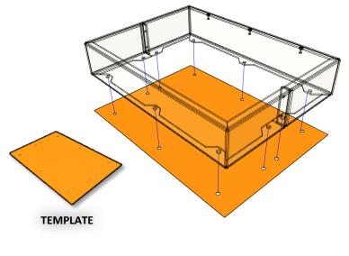
2.3 Secure the cabinet to the base with 3 screws located under the front door as indicated.
