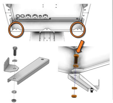
**1.3** Hoist the cabinet from the two lifting ears and slide it over the pole bracket. Secure the bottom bracket to pole with steel straps or screws.
