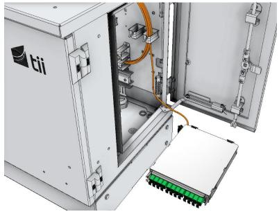
4.5 Slide the cassette back into place with the adapters facing the front of the cabinet. Once it is in position, secure it by pressing the push pin.
