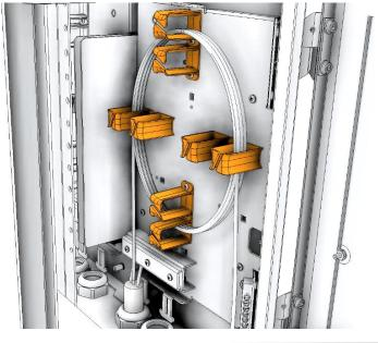
4.2 Insert cable thru any of the ports (2x per side), tighten external nut, secure jacket with hose clamp and fix strength member as indicated.
