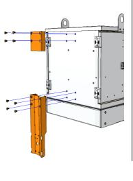
cabinet top. Install the pole bracket 4.25 inches below that mark, with screws or metal straps.
