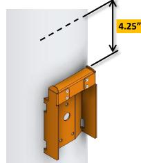
1.4. Attach Braces to holes on skirt with provided  $3/8'' \times 1''$  hex bolts and the split washers.
