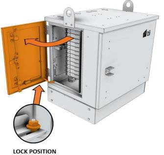
2.2 Slide cabinet over mounting base so the bracket at the back of the cabinet engages the lip of the base.
