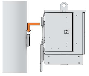
1.5 Attach L bracket of brace to the pole with provided 1/4" x 2" lag screws. Tighten the brace screws to secure position.
