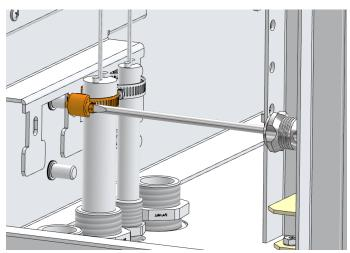
4.6 Lay strength member on back panel and clamp with provided bracket.
