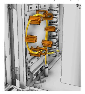
4.5 Insert distribution cable thru large cable port, tighten external nut and secure jacket with hose clamp.
