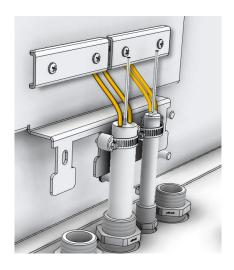
4.7 Remove packing material from behind the cassettes and discard it. Bring all fiber tubes out thru right side door.
