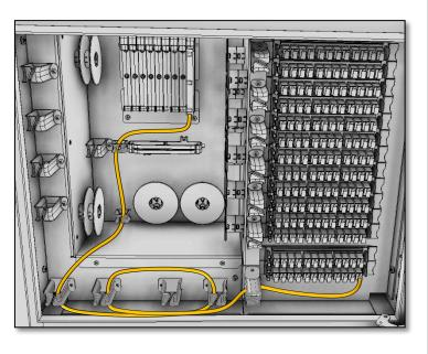
5.4 Connect splitter distribution legs to desired adapters on distribution field and route cable on provided management clips as needed.
