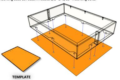
$2.2\,$  Slide cabinet over mounting base so the bracket on the back of the cabinet engages the lip of the base.
