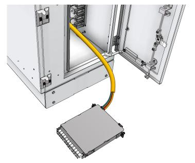
4.4 Store feeder cable slack on provided cable management clips. Mount feeder cassette back and secure in place with push pin.
