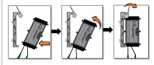
5.3 Connect splitter input legs to desired adapters on input area and route cable using the provided management clips as needed.
