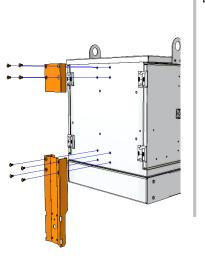
1.2 Mark on the pole the desired location of the cabinet top. Install the pole bracket 4.25 inches below that mark, with screws or metal straps.
