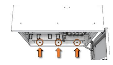
$3.2\,\,$  Bring grounding cable thru provided hole on bottom of cabinet, and securely fix to grounding bar.
