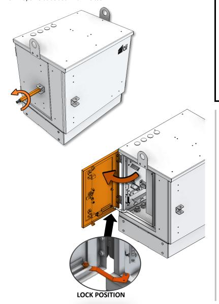
2.3 Secure with 3 screws from inside the cabinet as indicated above.
