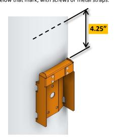
1.3 Hoist the cabinet from the two lifting ears and slide it over the pole bracket. Secure the bottom bracket to pole with steel straps or screws.
