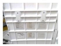
3. To divide door, remove 2 screws from door connector plate.
