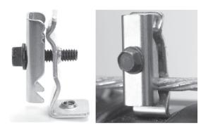
1.2 <u>ADSS Mount</u> – Optional mounting kit is designed for 10-15mm cable. Loosen hose clamp and thread through bracket slots and around cable. Tighten hose clamp to 40 in-lbs.
