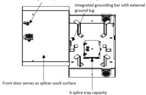
3 each top/bottom NPT ¾" compatible cable entry ports
