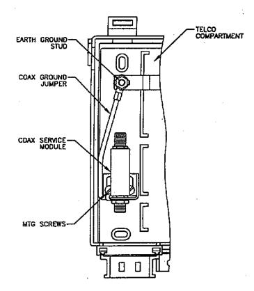
Installing Coax Service Module Into The Til 3500 Series BNID
