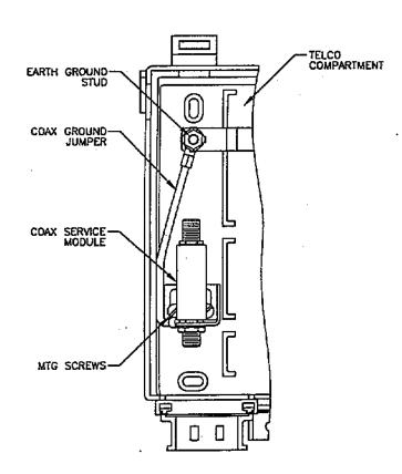
Installing Coax Service Module Into The TII 3500 Series BNID
