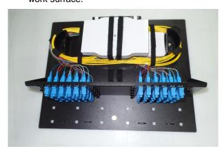
Remove master plate from front or rear to assist with fiber routing. Terminate or fusion splice feeder cable. Re install master plate with feeder cable. Store excess feeder in slack storage loop.
