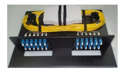
Remove master plate from front or rear to assist with fiber routing. Terminate or fusion splice feeder cable. Re install master plate with feeder cable. Store excess feeder in slack storage loop.
