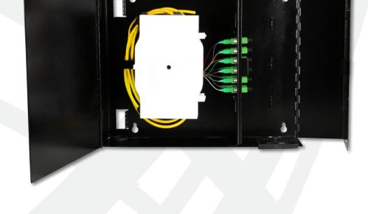
Wall mount fiber distribution unit designed to support patching and splicing in one unit. The enclosure has 2 adapter panel positions, allowing for a wide variety of fiber termination connector types. Two compartments separate the network terminations from the distribution terminations.
