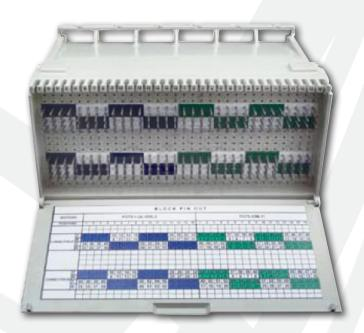
88 Equipment Terminal Blocks are used to terminate exchange equipment pairs on the horizontal side of a conventional main distribution frame (MDF) and provide a cross-connect field for jumpering to the Outside Plant (OSP) vertical side of the frame.
