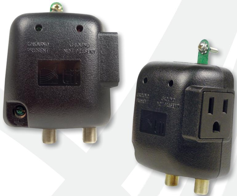
The 442CSE Grounding Module detects the presence of AC power and ground. It also provides an auxiliary AC receptacle designed with a side entry AC outlet and grounding for easy access to the unit and grounding connection through the ground tab. Two F-type female connectors provide the means of grounding the coax cable shield as well as signal integrity.
